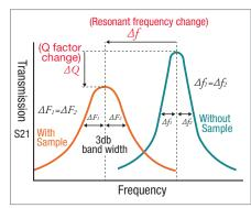
more, typical), even a slight change due to the insertion of a low loss sample causes a large Q factor change, which enables accurate measurements.
